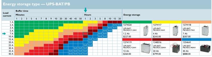
1+1 ... Two energy-storage types of the same capacity are required, based on ambient temperature of 20°C.
