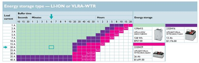
1+1 ... Two energy-storage types of the same capacity are required, based on ambient temperature of 20°C.
